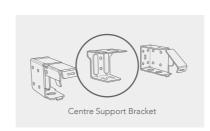
Open the gate of the box brackets and slide the headrail into position then snap the brackets closed.
