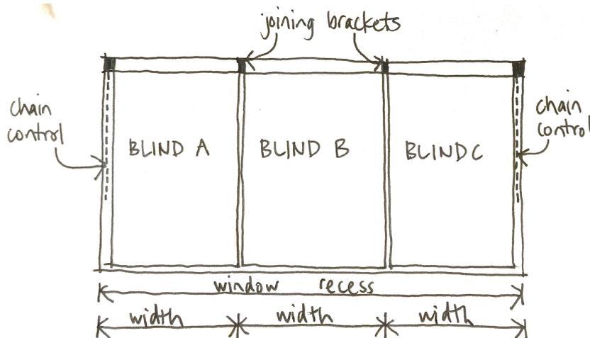
**Blind A** is operated by left side chain control. It has a 'linked' joining bracket and is coupled with Blind B on the right side.
