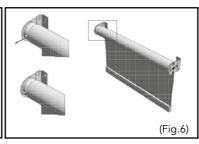
Then making sure the locating lugs on the end of the spring side is in the lowest position, place the blind into the spring end bracket. (Fig.5) Release the pin (do not pull all the way out) from the front side of the spring. Your blind has been pre-tensioned and is now ready to operate and will stop at the desired top position. (Fig.6)
