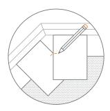
2 Hold the two pieces of card against the corner of the bay so that the two marked lines meet.
